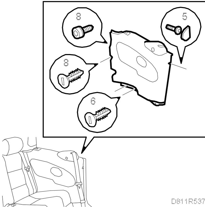
6. Remove the plastic screws which secure the trim to the lower edge.
