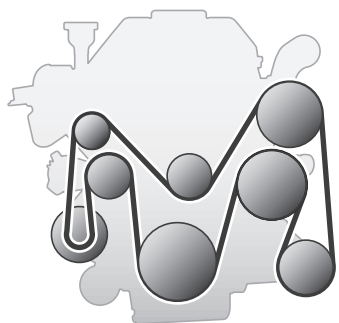
Drive belt, 4-cylinder with A/C system
