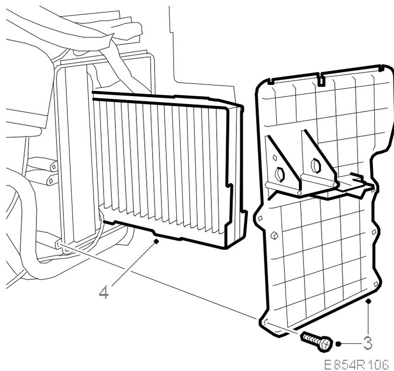
4. Remove the fresh-air filter and filter element or particle filter.
