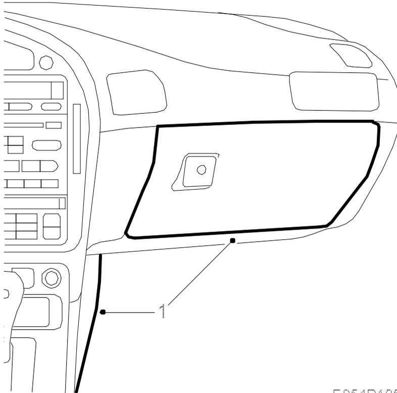
2. Cut off the cable ties securing the wiring harness to the service cover. Cut also the cable tie holding the cooler hose to the glove box.
