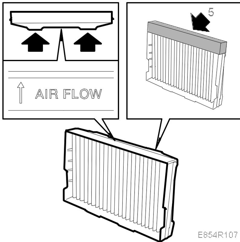
6. **Cars with retrofitted A/C:** Break off the plastic lugs on top of the filter.
