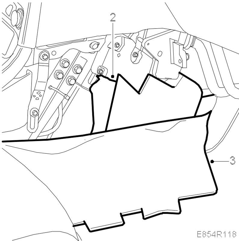
3. Fit the carpeting to the centre console on driver and passenger sides.
