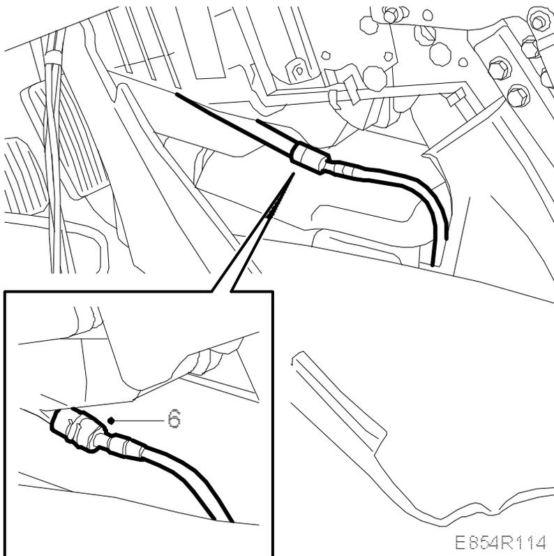
7. Blow compressed air through the hose, with the hose pointing towards the floor.
