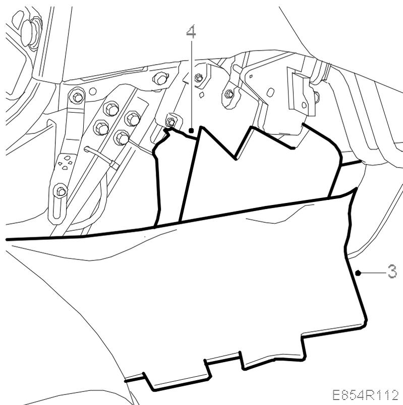
4. Remove the insulation from the passenger side.
