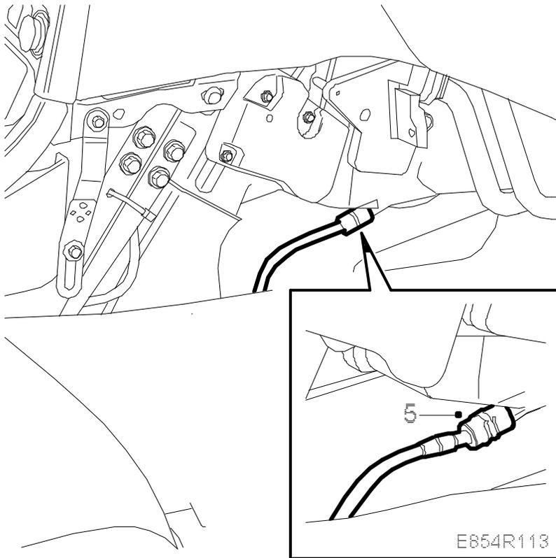
6. Remove the hose clip from the driver's side. Remove the drainage hose from the heating and ventilation unit.
