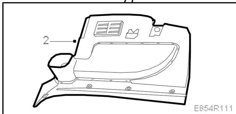
2. Remove the sound insulation from driver and passenger sides.
