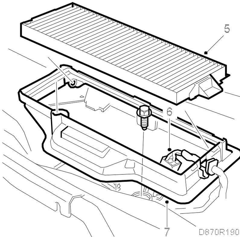
6. Unplug the ventilation fan electric connector.
