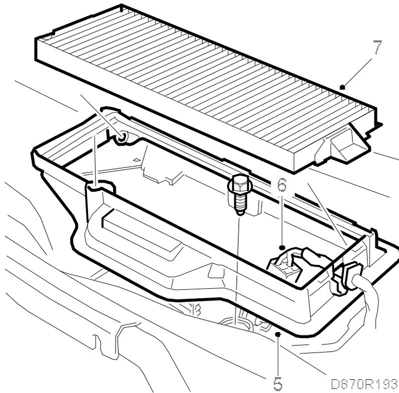
6. Plug in the ventilation fan connector.
