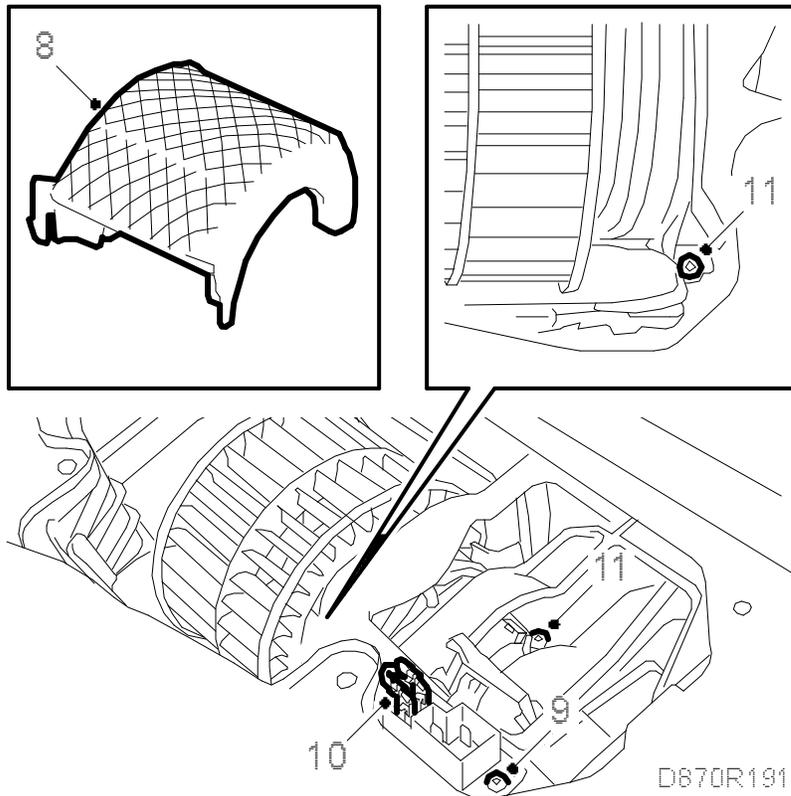
9. Remove the bolt that secures the electric connector.
