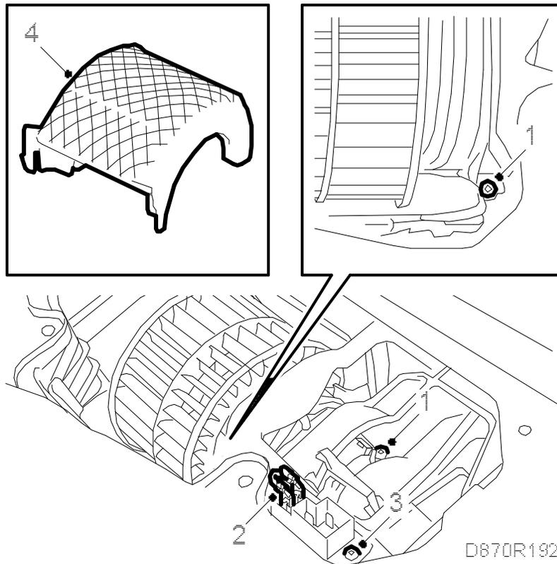
1. Fit the ventilation fan and tighten the bolts.
