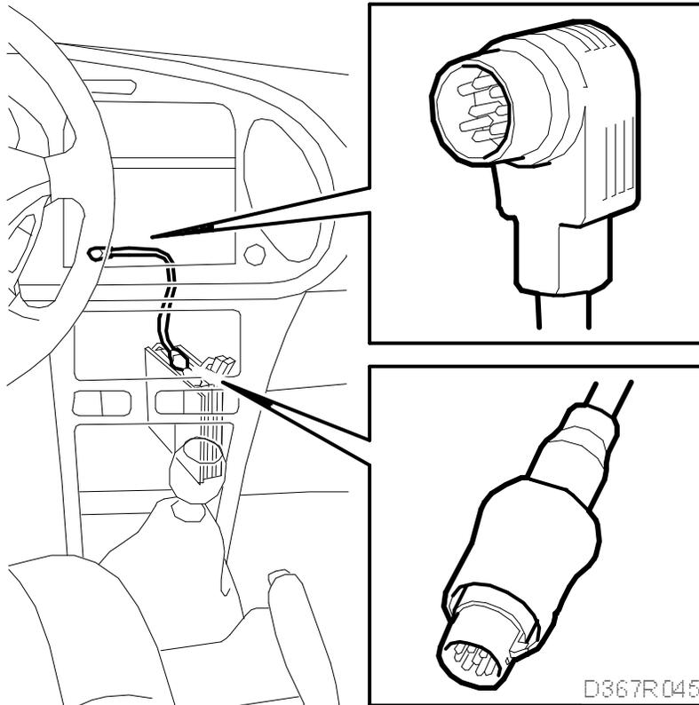
1. Remove the glove box and the side panel on the right-hand side of the centre console.
