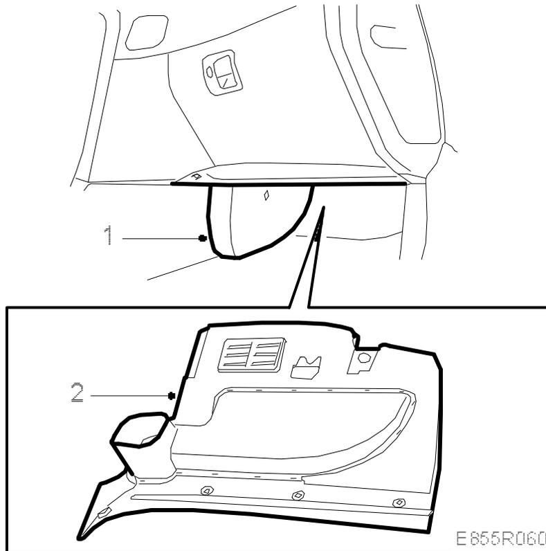
1. Remove the cover for the heating and ventilation unit.
