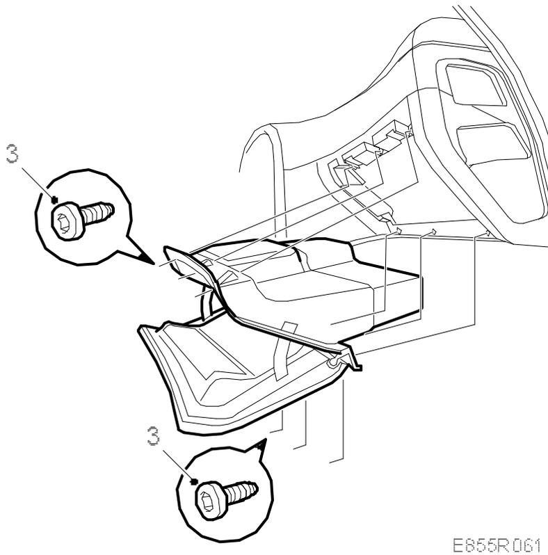
4. Undo 3 retaining screws underneath and 3 retaining screws inside the glove box.
